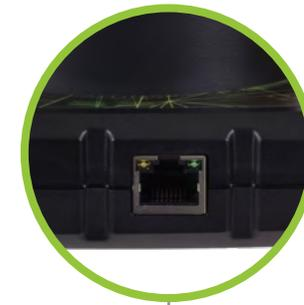
Via an orange and a green LED you can see whether the CIP is successfully connected to the Car Lock Systems server.
