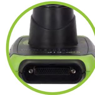
Use an OBD cable to connect the CIP to any vehicle. Now follow the instructions in the **CIP quick start manual** to connect to Car Lock Systems.
