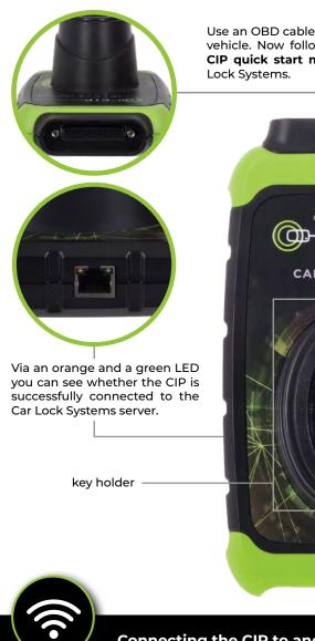
Use an OBD cable to connect the CIP to any vehicle. Now follow the instructions in the **CIP quick start manual** to connect to Car Lock Systems.
